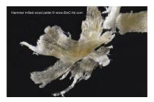
Figure 3. Particle from wood pellets milled in a hammer mill.
