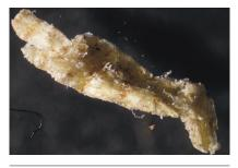
Figure 4. Particle from wood pellets milled in a vertical spindle mill.
