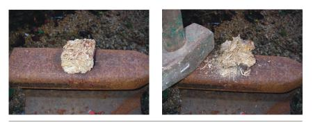
Figure 2. A briquette of biomass before and after being hit by the same sledge hammer.
